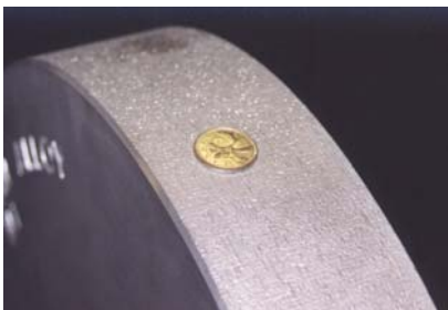
Surface quality of 458-mm M1 billet cast using Hatch Hot Top Casting Technology
