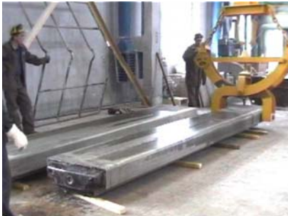
Magnesium T-Bar cast using Hatch Hot Top Tooling technology, at the AVISMA facility; Berezniki, Russia
