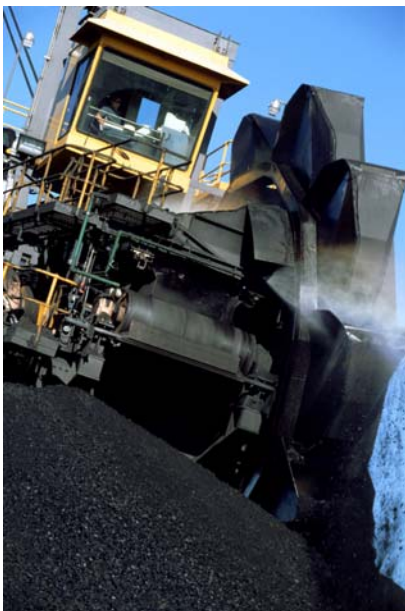
Stockpile capacity and layout are key to determine capital cost and component capacities. For the Dalrymple Bay Coal Terminal 7X in Australia, Hatch used simulation tools to optimize the stacker reclaimers
